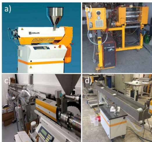
Figure 1: The compounding platform in CSEM. a) Extruder; b) Flat film line; c) Compounder; d) Pelletizer.
