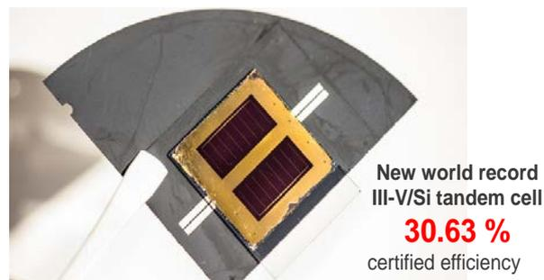
Figure 2: Picture of 1 cm² III-V/Si tandem cells mechanically stacked, demonstrating up to 30.63% record efficiency.
