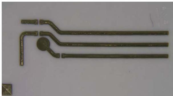
Figure 3: Printed electronic features on nanoporous paper.
