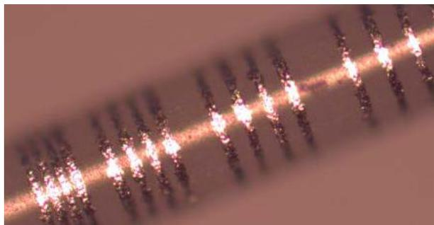
Figure 2: Printed electrodes or antennas on plastic rods.
