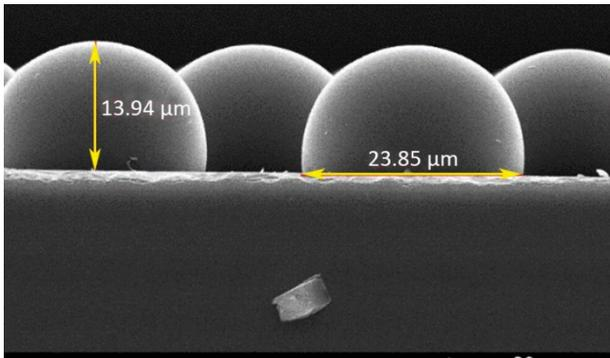
Figure 1: SEM image of more than hemispherical microlenses produced by reflow—cross-section view.
