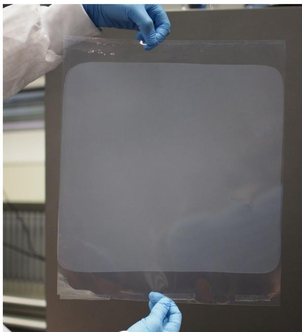
*Figure 1: Photograph of a 300 × 300 mm<sup>2</sup> sample. The nanoimprinted structures give a milky aspect to the substrate. The final thickness of the textured foil is 130 micrometers.*
