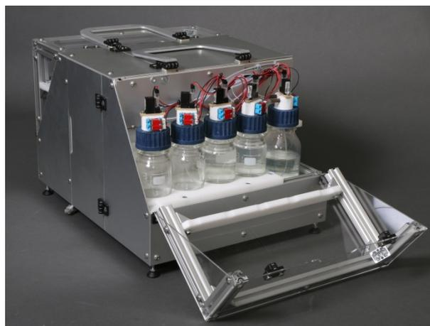
Figure 2: Food quality monitoring system integrating a controlled, pressure driven dispensing subsystem (all five bottles are controlled).
