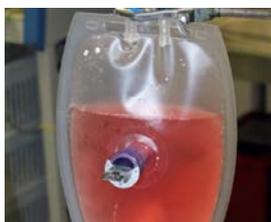
Figure 2: Biosensor integrated in a single use bioreactor [2].
