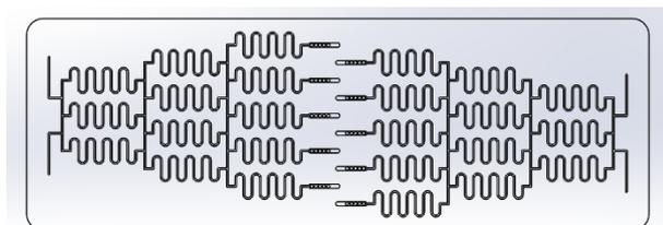
Figure 1: CAD drawing of the microfluidic chip with a gradient generator and spheroid traps in the center. Dimensions of the chip are 75 × 25 mm.
