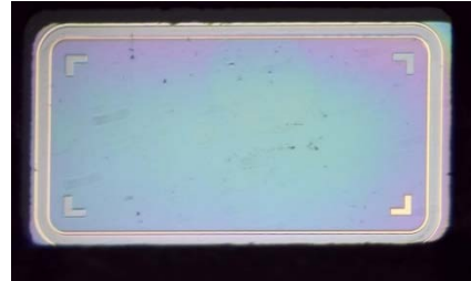
Figure 2: Hermetically sealed glass on silicon package.
