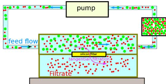
Figure 4: Working principle of the micro-fluidic filtering system.
