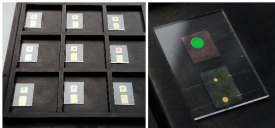
Figure 2: Planar waveguides with three diffractive gratings each.
