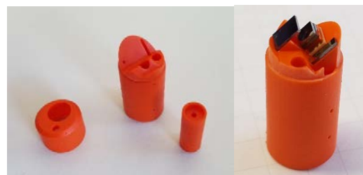
Figure 4: Endoscope head prototype.
