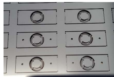
Figure 3: MEMS scanner with integrated focus.
