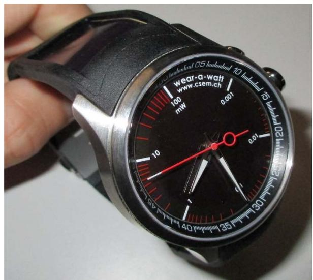
Figure 2: Wearable prototype with thin-film PV cells integrated in the wristband (2016). The cells are put on both parts of the plastic wristband and cover an area of 2.0 × 4.5 cm<sup>2</sup>. From indoor to outdoor the light intensity typically varies typically by 3 orders of magnitude which is why the milliwatt units are represented on a logarithmic scale on the watch dial (white and red tick marks) instead of the usual hour ticks.
