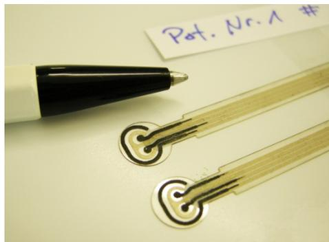
Figure 2: Screen-printed dual electrode sensors for multiple parameter monitoring
