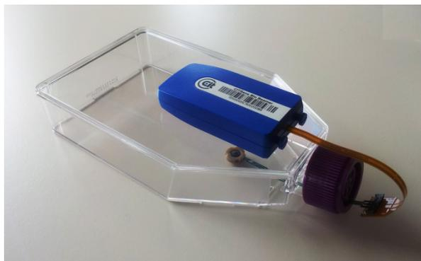
Figure 1: The online cell culture monitoring system CITSens Bio, adapted for the use in a T-flask.
