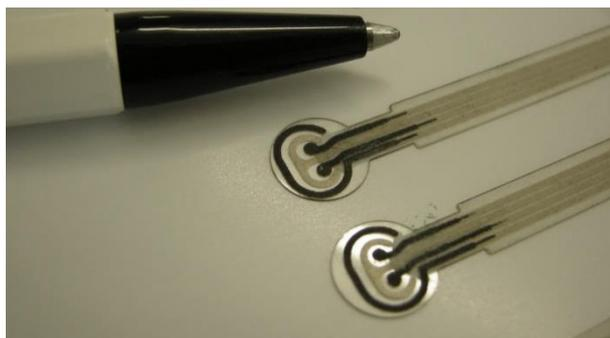
Figure 2: Screen-printed dual electrode sensors for multiple parameter monitoring.
