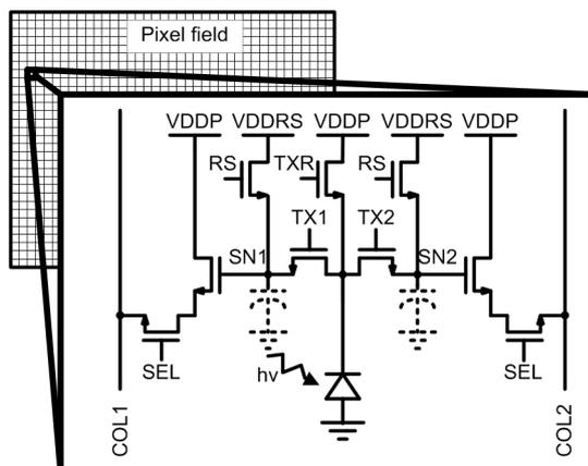
Figure 1: Schematic of the pixel
