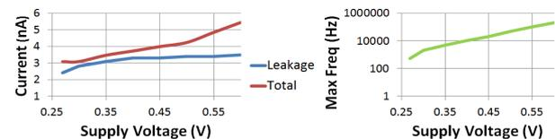
Figure 2: SRAM leakage, total current and maximum frequency.
