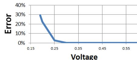
Figure 3: SRAM measurements for bit errors degradation.
