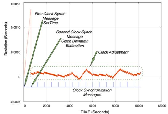
Figure 2: Clock adjustments under ambient temperature conditions.
