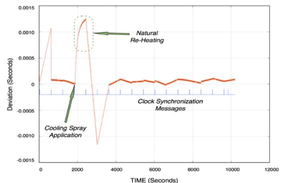
Figure 3: Clock adjustments under variable temperature conditions.
