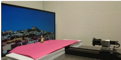
Figure 1: Our acquisition setup composed of a motorized linear stage, a motorized turntable, a background screen and a uniform colored ground.
