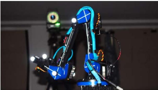
Figure 1: Robot arm with mounted reflectors and IMUs.
