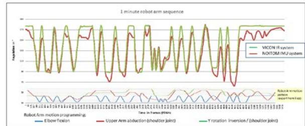
Figure 3: One minute angular data sequence showing deviation patterns between Vicon and Noitom systems.
