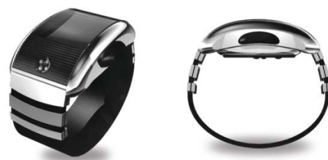
Figure 2: Health watch prototype developed at CSEM for the monitoring of motion related and cardiac activity parameters.
