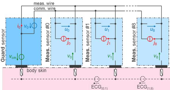
Figure 1: ECG12CS circuit with 1 guard and 9 measuring sensors.
