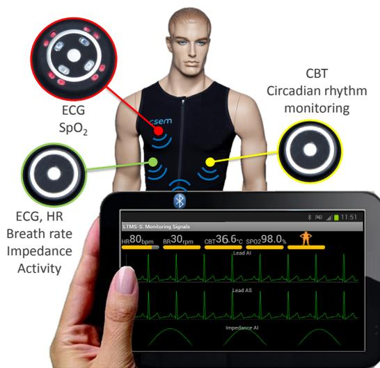
Figure 1: Overview of LTMS-S monitoring capabilities.
