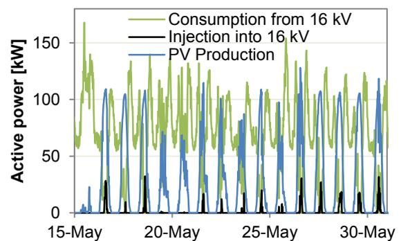
Figure 2: Net power consumption and injection from the low-voltage (seven feeders) to the medium-voltage level, and the production of a 145 kW<sub>p</sub> PV system connected to one of the feeders.
