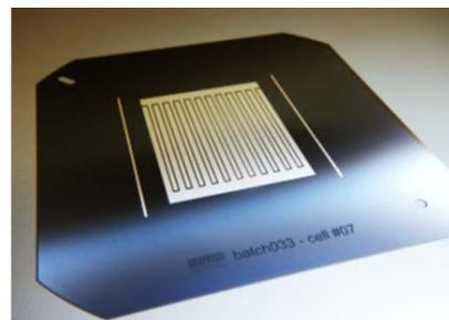
Figure 3: View of the back side of a 3 x 3 cm<sup>2</sup> IBC SHJ solar cell fabricated at CSEM-EPFL. The interdigitated pattern of the p and n contacts is clearly visible.
