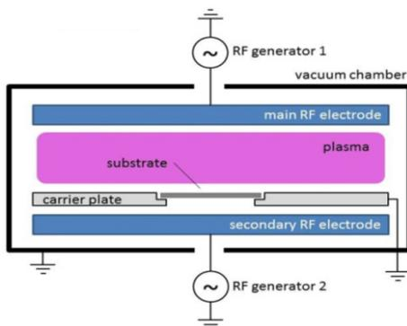
Figure 1: Schematic design of the Mirror PECVD reactor. A sister chamber with inversed position for the main and the secondary electrodes is used for deposition on the other side of the substrate.
