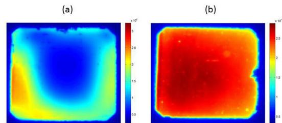
Figure 2: Photo-luminescence imaging of SHJ solar cell precursors produced in the Mirror reactor (a) without power compensation; (b) with power compensation.
