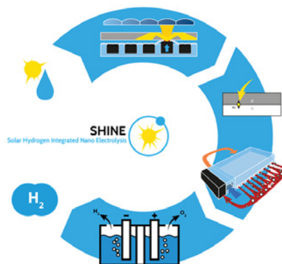
Figure 1: Conceptual view of the four elements of the integrated PEC device to produce hydrogen from solar energy and water [1] [5] [6] .
