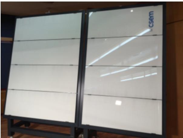
Figure 1: White PV modules fabricated at CSEM.
