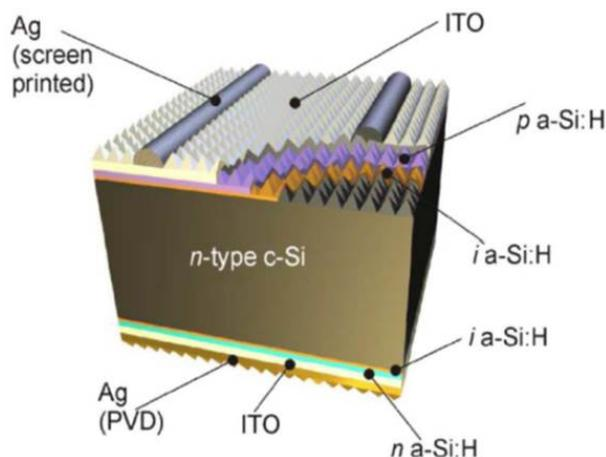
Figure 1: Schematic representation of a silicon heterojunction solar cell.
