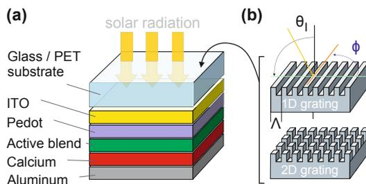
Figure 1: (a) Standard device architecture of an OPV. (b) A sub-micrometer line grating (1D) or crossed grating (2D) is fabricated at the light incident surface of the device.
