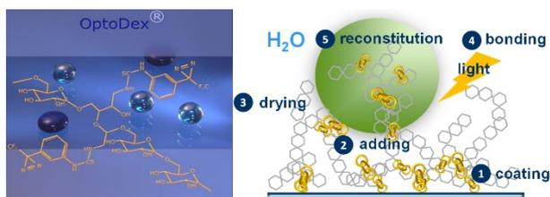
Figure 1: Schematic of the OptoDex® technology: ① Adsorptive coating of surface with photolinker polymer; ② Addition of biomolecules; ③ Stress-less vacuum drying in OptoDex® embedding; ④ Dry state bonding by photoactivated linking polymers; ⑤ Rehydration reconstitutes functional biomolecule.
