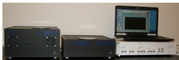
Figure 2: Complete UV absorption and MALS detector system for nanoparticle analysis. The lock-in system used for MALS detection is visible on the right.
