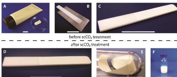
Figure 1: Model sunscreen at different stages before (A–C) and after (D–F) the novel supercritical CO<sub>2</sub> treatment. Scale bars are 25 mm.
