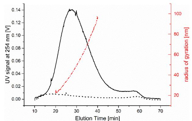
Figure 2: Elugrams of the TiO<sub>2</sub> spiked (solid line) and blank (dotted line) model sunscreens, after scCO<sub>2</sub> treatment and resuspension in water. The red line shows the radius of gyration measured by MALS.
