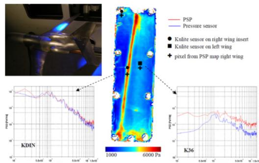
Figure 2: RMS map and PSD from nano-PSP (Insert #3). Pressure  $P_{i0} = 185\text{ kPa}$ , speed  $M = 0.875$ , incidence  $\alpha = 1.11^\circ$ , acquisition frequency  $F_{acq} = 5000\text{ fps}$ . Photograph of the insert on the model.
