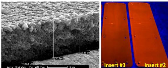
Figure 1: (Left) SEM micrograph of the nanoporous silica layer cross-section of a sample similar to insert #3 (10  $\mu\text{m}$  thick); (Right) Fluorescence pictures (excitation 365 nm) of nano-PSP homogeneously treated inserts #2 and #3.
