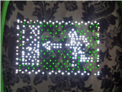
Figure 1: 400 assembled LED's showing EXIT sign.
