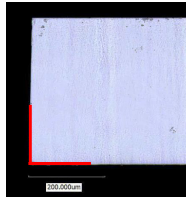
Figure 2: TruMicro IR manufactured Silicon cutting edge with a taper angle of 90°.
