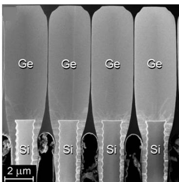
Figure 1: Cross-section view SEM micrograph of Ge three-dimensional crystal array grown on pillar-patterned Si substrate [2].
