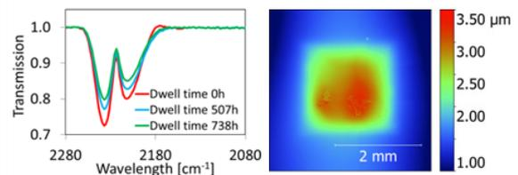
Figure 3: FTIR  $\text{N}_2\text{O}$  absorption spectra in the cavity (left) and deformation of the membrane (white light interferometry) (right).
