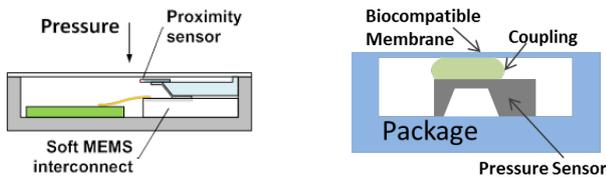
Figure 1: Thermal proximity (left) & mechanical coupling (right) pressure sensing concepts.
