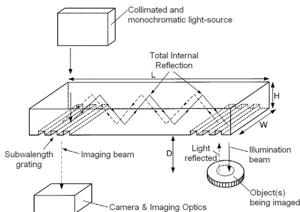
Figure 1: Sketch of a slab waveguide diffractive endoscope.
