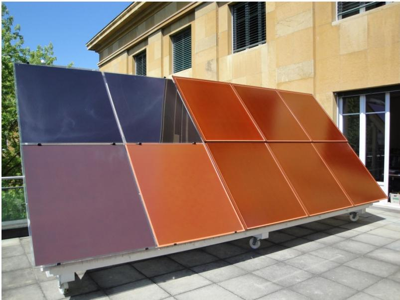
*Tile-colored photovoltaic panels – Archinsolar Project with EPFL's PV-Lab, Neuchâtel. CSEM has already brought out a first series of 150 modules. © CSEM 2014*
