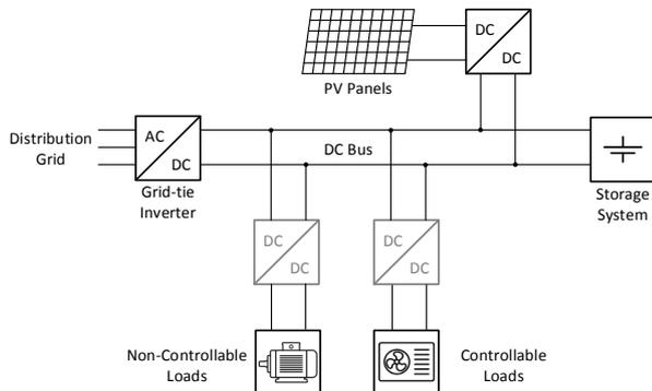
Figure 1: Electrical architecture of the microgrid.
