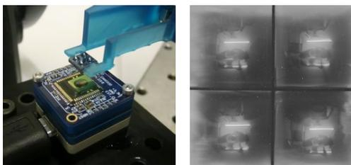
Figure 2: Lens array prototype during assembly on CMOS imager (left) and resulting 4 pictures (right).
