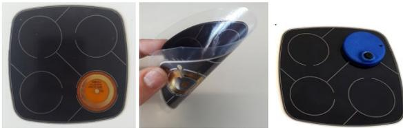
Figure 1: Front side view of the PV cell with the magnetic dock (left) cell flexibility (middle) and camera docked on PV (right).
