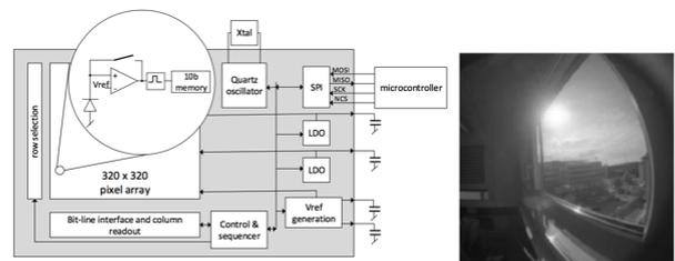
Figure 4: Chip architecture (left) and resulting image (right).
