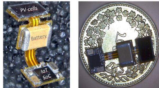
Figure 2: Photographs of the energy autonomous miniature IoT WSN.
