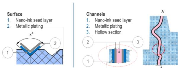
Figure 1: Cross sections of the geometries to be functionalized and illustration of the plated seed-layer. The outer surface has the shape of a V-groove roaming the perimeter of a cylinder. The channel is inside the structure.
