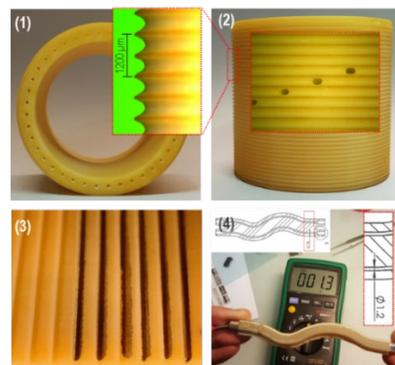
Figure 3: (1) & (2) 3D printed SRA prototype, (3) V-grooves plated ink layers, (4) channel test sample electrical resistance measurement.
