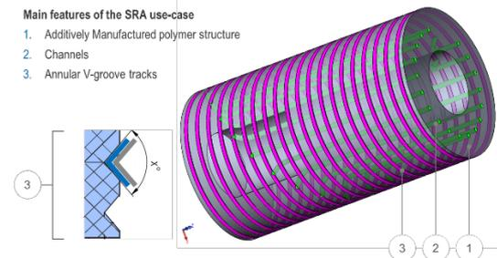
Figure 2: Pre-design of the SRA use-case with its main features.
