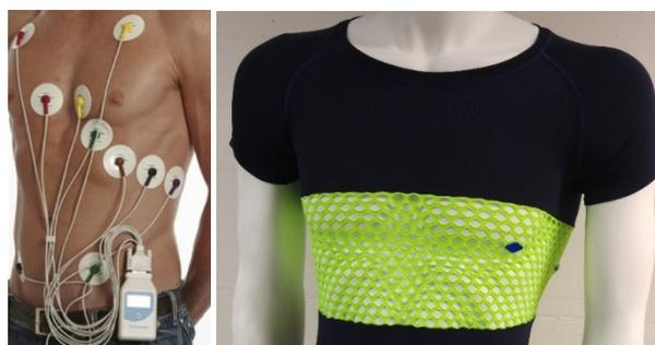
Figure 1: Classical solution (called Holter) to measure medical multi-lead ECG (left) and wearable solution with dry-electrode cooperative (right) showing a mock-up of the targeted wearable (button sensor inserted in an electrically conductive mesh allowing free positioning of sensors).
