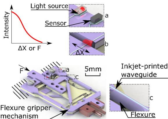
Figure 1: Combining flexure mechanisms, e.g., a flexure gripper mechanism, together with inkjet-printed wave guides for intensity based sensing of displacement ( $\Delta X$ ) or force ( $\Delta F$ ).
