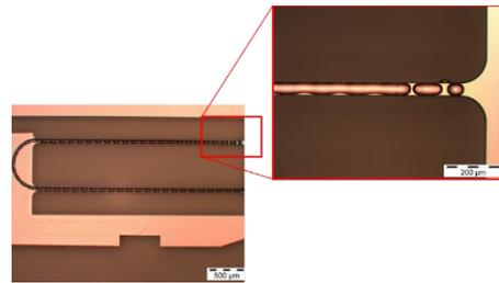
Figure 2: Waveguide printed on top of narrow 50 micron Si beams.
