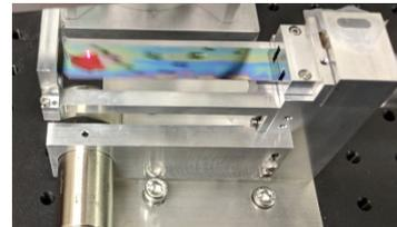
Figure 3: A custom designed opto-mechanical fatigue measurement setup with a silicon flexure moved for  $1e7$  cycles.
