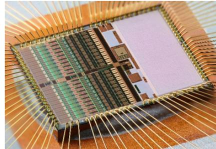
Figure 1: DeTOP system on chip micro-photograph (3 x 3.7 mm<sup>2</sup>).
