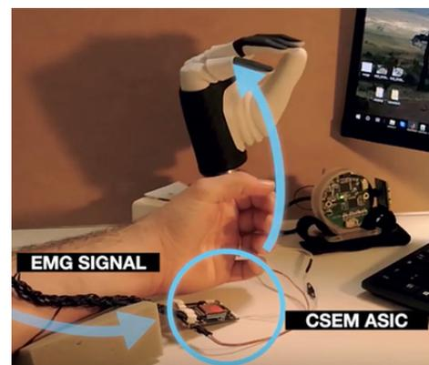
Figure 3: Prosthetic hand control using DeTOP system on chip (CSEM ASIC).
