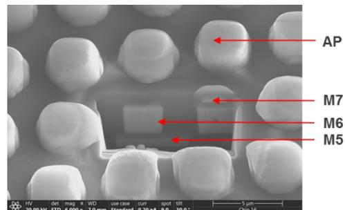
Figure 2: Cross section from FIB showing precise milling up to metal M5 layer while only touching inactive M6 and M7 layers.
