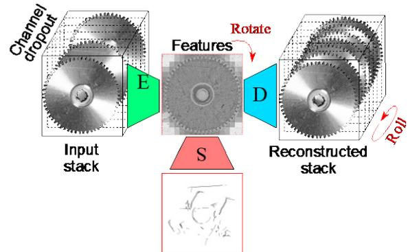
Figure 2: Rotate & Roll Channel Auto-Encoder architecture: Encoder (E) extracts the features, Decoder (D) estimates the original images, and Detector (S) segments the defects.
