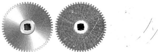
Figure 1: Defect detection of a watch part. (left) One of the many input images, (middle) Extracted features; (right) Defect predictions.
