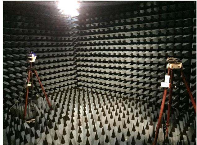
Figure 2: Measuring setup in the anechoic chamber.
