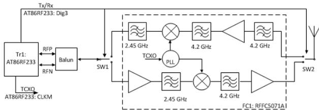
Figure 1: WAIC architecture using two switches.
