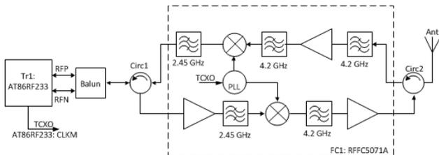
Figure 2: WAIC architecture using two circulators.
